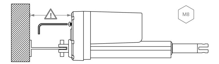
The torque required to manually move the extension tube is within 1.7 Nm, maximum 65 RPM. Please do not run the outer tube to the end of stroke as that may damage the actuator.
