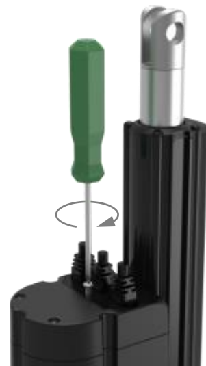
Step 6: Re-screw with the torque approximately 1.5Nm.
