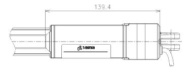
B. Dimensions - Standard for Load and Speed Code K, J, G (mm)
